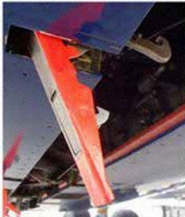
(d) Cowls open on hold open device, latch handle hook disengaged. Cowling not locked.
