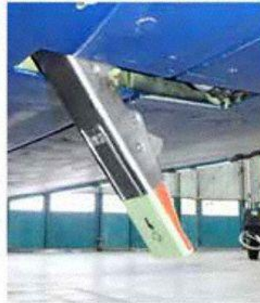
(c) Latch unlocked, latch handle hook disengaged. Cowling not locked.
