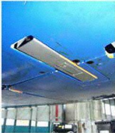
(a) Latch locked, cowling locked.
